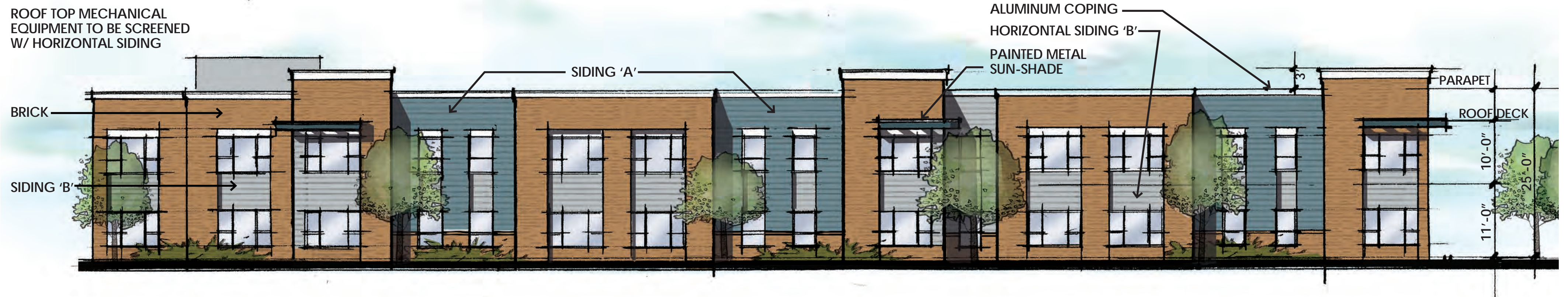
2 NORTHEAST ELEVATION (OUTER DRIVE) 3/32" = 1'-0"
