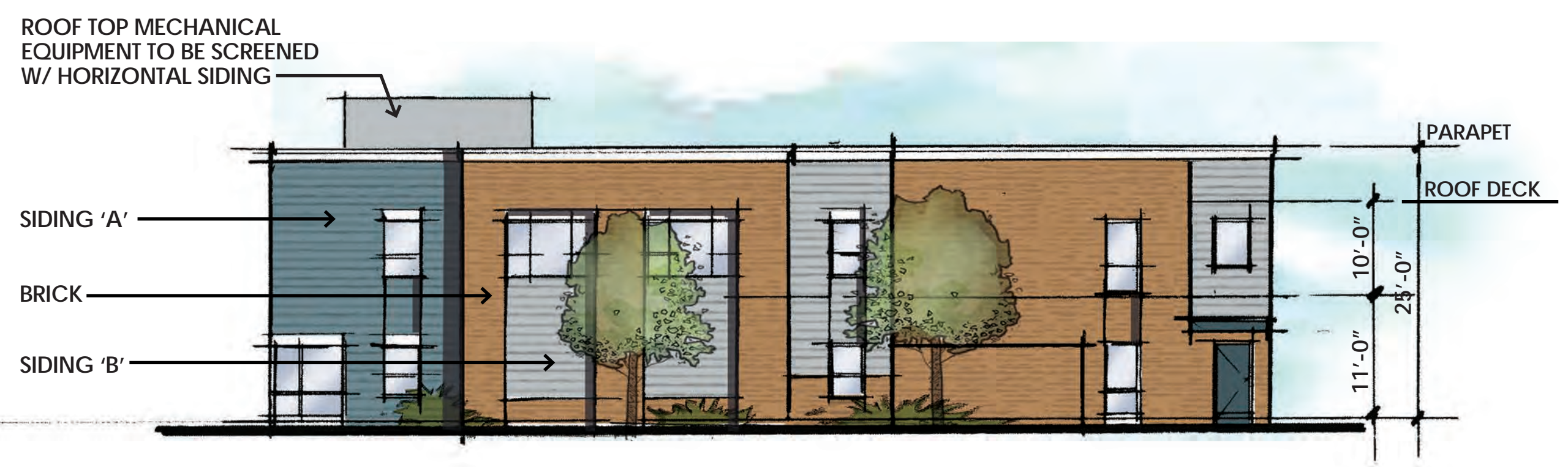
5 SOUTHEAST ELEVATION (FACING PARKING LOT) 3/32" = 1'-0"
